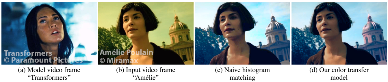
Figure 5: We would like to transfer the color palette of the model video frame (a) to an input video frame (b). (c) The simplest way to do this would be to apply histogram matching in each color channel (and the foreground and background) independently. While this might match the color styles, it often produces artifacts (note, the color artifacts on Amélie’s face). (d) Our color transfer model is able to produce an equivalent result without any artifacts. Video credits: “Transformers”(2007) ©Paramount Pictures (model), “Amélie”(2001) ©Miramax Films (input).
